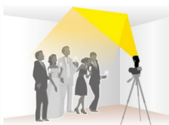
Fig. 2: Bounce flash with on-camera flash is possible if the flash can rotate up and down (bounce) and to the sides (swivel), left. The idea is to bounce the flash off the ceiling or the walls (including the wall behind the photographer, see below). This distributes the flash over a larger area, softening the light and reducing the light fall off. When it is possible, it can result in very pleasant portraits, group pictures, or pictures of rooms and interior spaces. Some flashes have a small card called a "catch eye card" (right) which helps put a sparkle in the subject's eyes.
